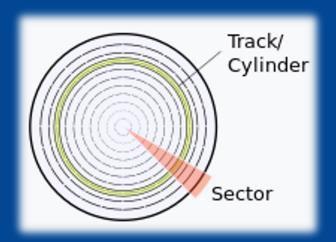
The information is recorded in bands; each band of information is called a track. Each platter has the same number of tracks and a track location that cuts across all platters is called a cylinder.
